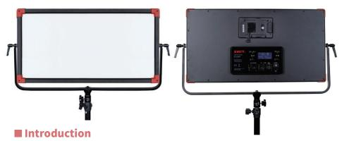
PL-E90D is specially designed for field portable lighting applictions. 480pcs SMD-LEDs are mounted in the inner edge of the light frame, and with SWIT unique 90° light guide technology, PL-E90D can output bright, soft and equally spread light, meanwhile, the light body is slim enough and portable, which is an ideal light source for interview kit and field video productions. There are two communication control modes: DMX communication mode and interaction control mode.
