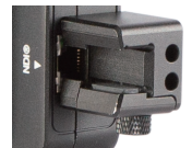
The clamp to fix RJ45 network cable
