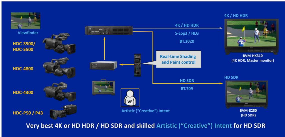
Figure 3: Image of SDR-based camera shading
