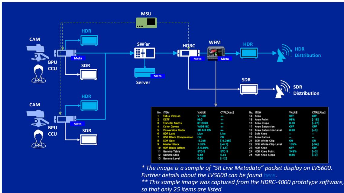
Figure 7: How SR Live Metadata travels through a production system and can be monitored
