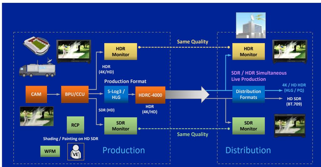
Figure 2: Image of simultaneous HDR and SDR production by one single system and crew
