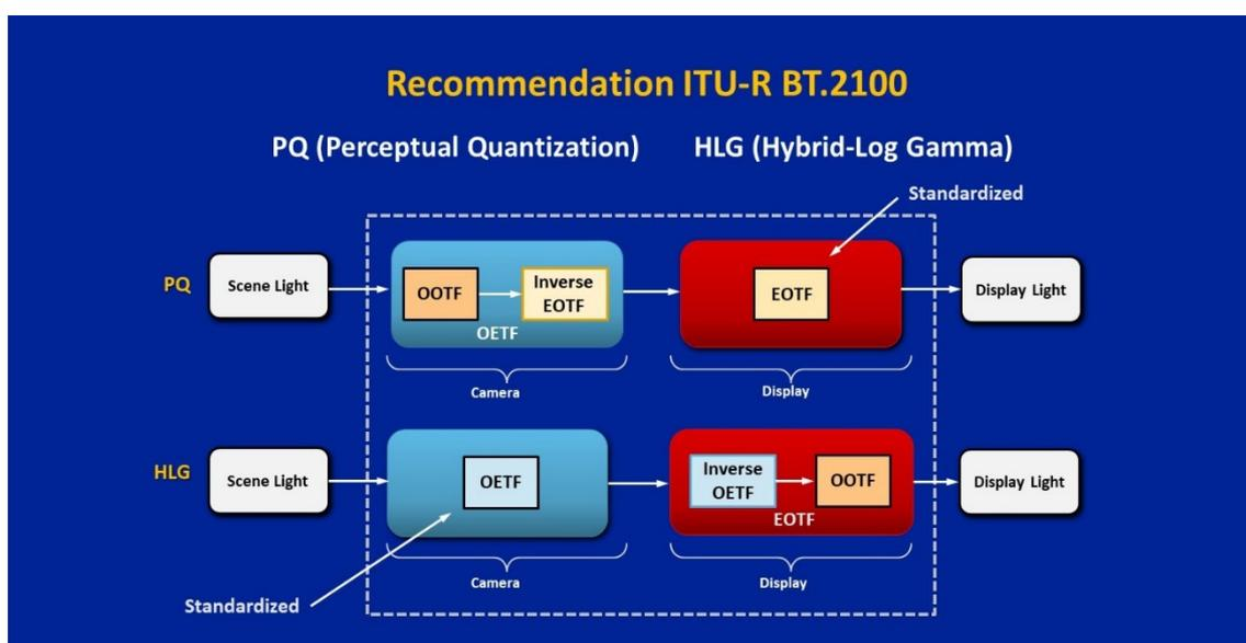
Figure 20: Processing diagrams of HLG and PQ
