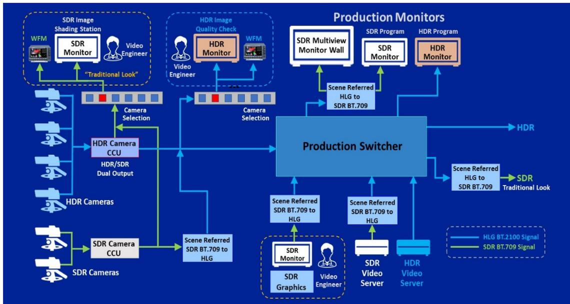
Figure 13: Scene Referred-based HDR/SDR simultaneous production
