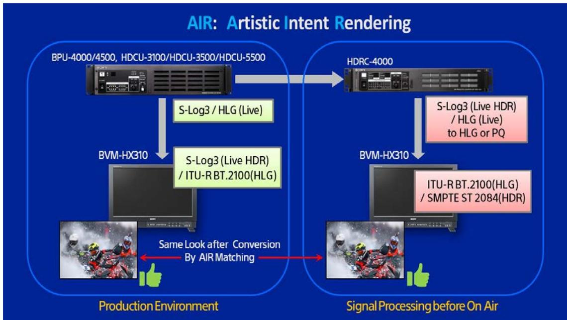
Figure 4: How AIR Matching works
