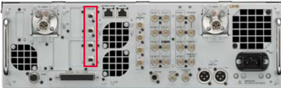
HDCU-5000 Rear view with the optional HKCU-SDI50
