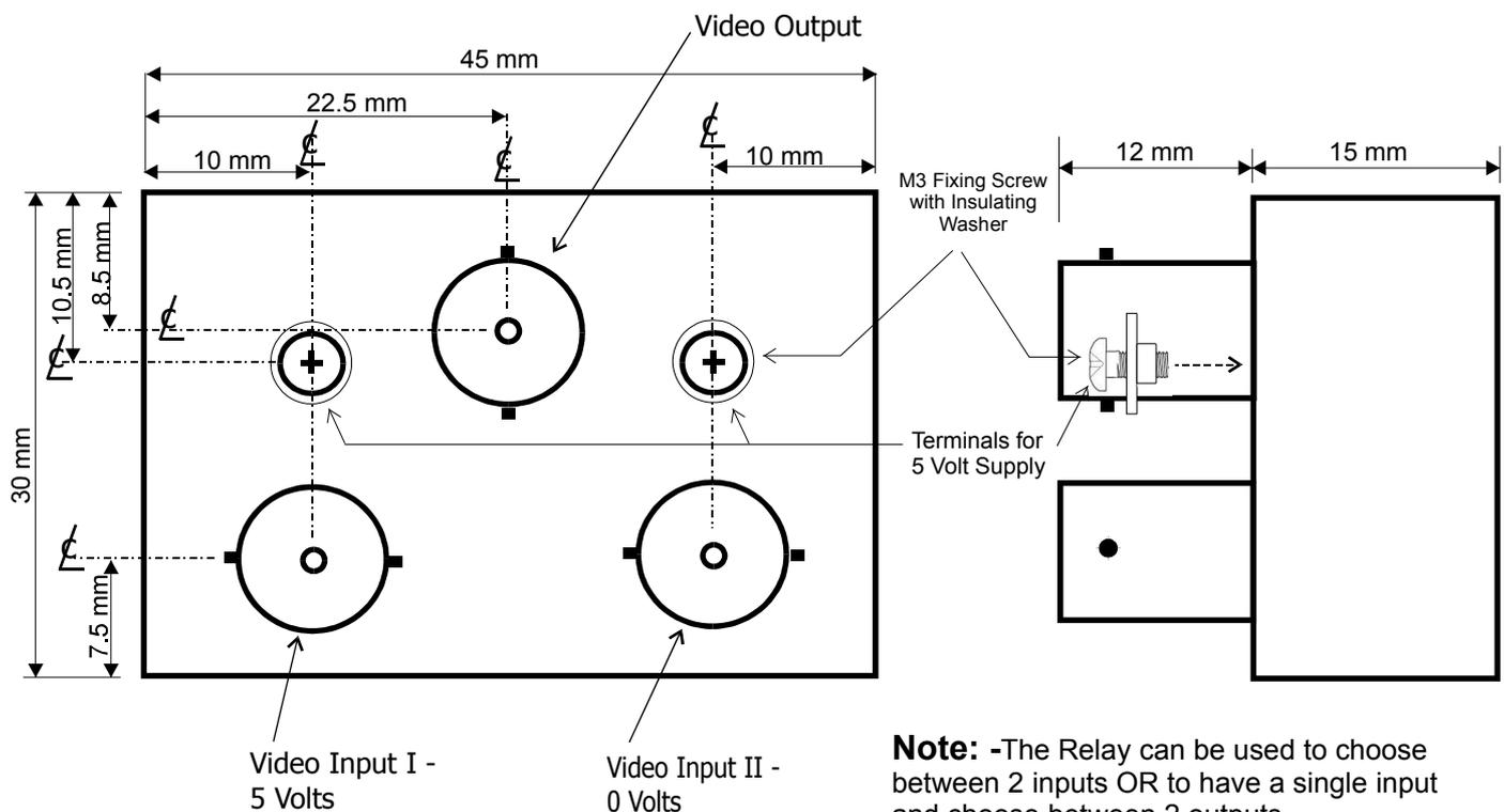
**Note:** -The Relay can be used to choose between 2 inputs OR to have a single input and choose between 2 outputs.
