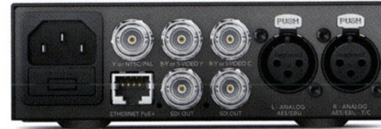
Teranex Mini - Analog to SDI 12G Convert YUV/S-Video/Composite with analog or AES/EBU audio to SD, HD and Ultra HD SDI.
