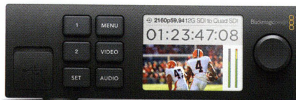
Teranex Mini Smart Panel Optional front panel with built in color LCD screen and push button controls for adjusting settings, seeing menus and monitoring conversions.
