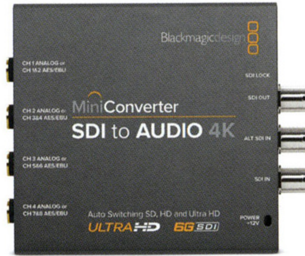
Mini Converter SDI to Audio 4K De-embed audio to 8 ch AES/EBU or 4 ch analog audio in SD, HD or Ultra HD.
