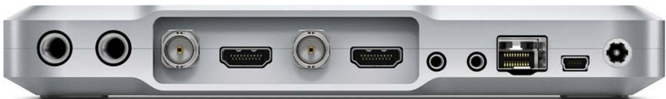
Connect to analog audio mixers using the de embedded audio outputs.
