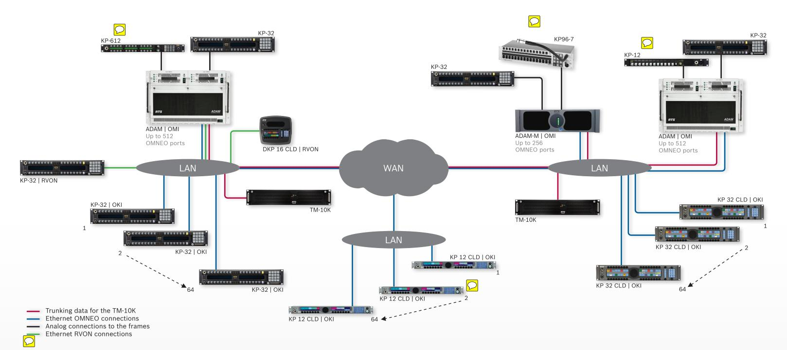
RTS+OMNEO media networking supports a PURE IP network infrastructure. Deploying a new RTS intercom solution has never been easier: an entire ADAM system can now be connected via OMNEO. Systems can be trunked together and user stations can be deployed all over standard Ethernet hardware. With the inherently high audio quality and low latency of the OMNEO connection, OMNEO links can be employed anywhere there is sufficient network bandwidth.
