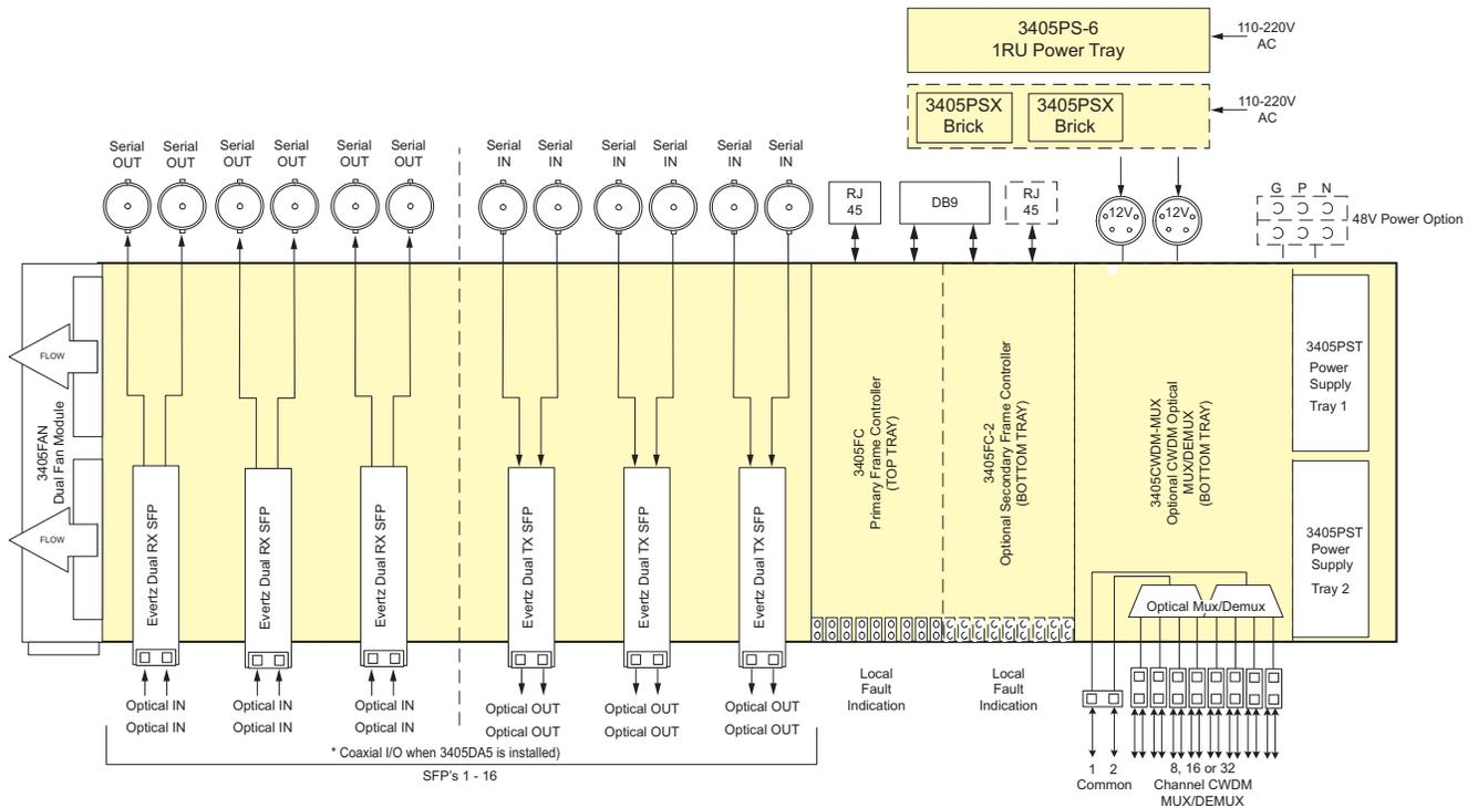
\*\*Note: Optional redundant frame controller (3405FC-2) cannot be used simultaneously with the 3405CWDM series units
