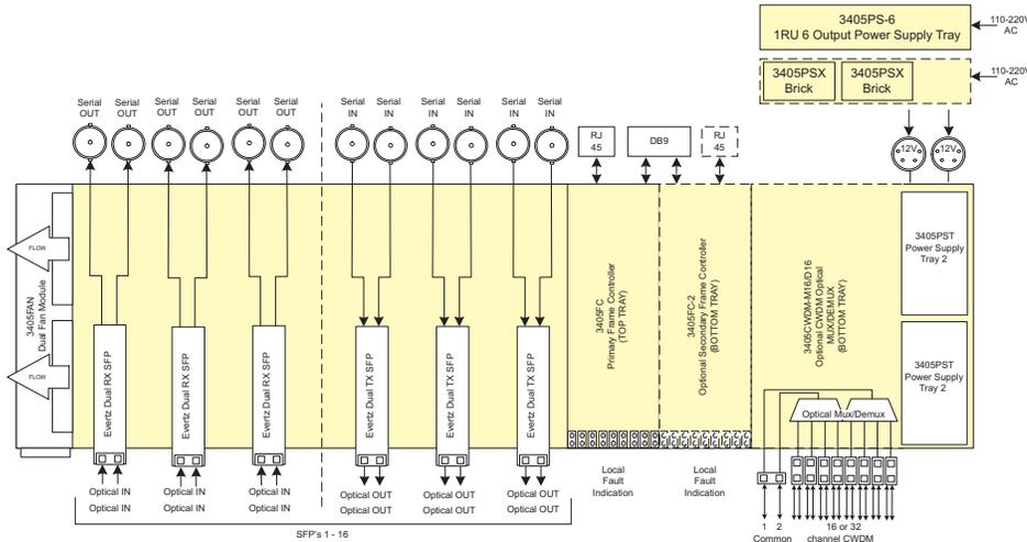
\*\*Note: Optional redundant frame controller (3405FC-2) cannot be used simultaneously with the 3405CWDMM-16/D16 unit
