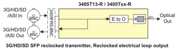
The Evertz® 3405FR-BNC SFP frame is the ideal solution for today's low cost, high density fiber optic distribution needs. The 3405FR-BNC provides the flexibility to handle the high-speed requirements of 3G and HDTV as well as SD-SDI, SDTi, and DVB-ASI.
