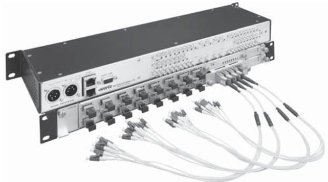
Numerous parameters such as optical power and electrical signal presence and rate can be accessed remotely to monitor system integrity. The 3405FR-DIN was designed to provide carrier-grade reliability with all SFP's, power supplies, frame controllers and the fan module being hot-swappable. There are no active components in the frame itself, a patent-pending feature from Evertz ensuring that the frame and coaxial cabling never need to be removed from the rack for service.
