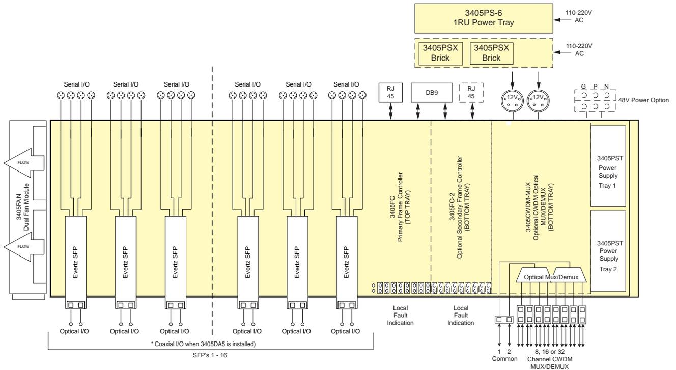
\*\*Note: Optional redundant frame controller (3405FC-2) cannot be used simultaneously with the 3405CWM series units
