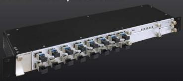
Evertz® 3405FR is the ideal solution for today's low cost, high density fiber optic distribution needs, providing flexibility to handle the high-speed requirements of 3G & HDTV as well as SD-SDI, SDTI, and DVB-ASI.
