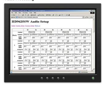
The Mini Master Control Switchers incorporate the latest in audio processing. Source selection is defined on an input-by-input basis. Each input can be either embedded or discrete as each unit has support for 8 channels of associated audio. Transition switching from embedded to discrete inputs is married to the video transition rate and handled internally by the system processor.
