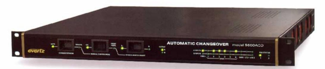
The 5600ACO offers connections for 6 color black, (or tri-level sync signals), 10MHz and DARS. Each 5600MSC Master offers two LTC outputs that may be used for different timecodes. All four LTCs are fed to the 5600ACO on two 'D' connectors, one for each Master. The LTC outputs from the selected master are available on two XLR connectors on the 5600ACO.
