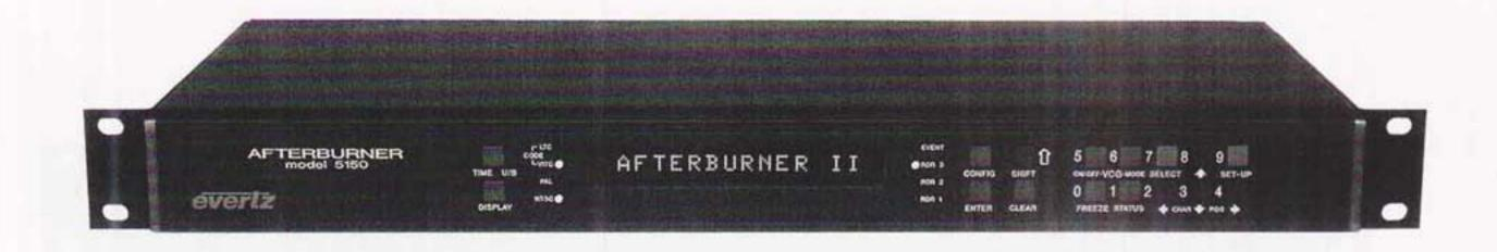
The 5150 Afterburner is a full featured Analog VITC and LTC Time Code Reader, VITC to LTC Translator with a full function Character Inserter. The Afterburner reads SMPTE RP201 3 line VITC and displays field accurate video and audio time code as well as KeyKode and 3:2 pulldown on material transferred from film.
