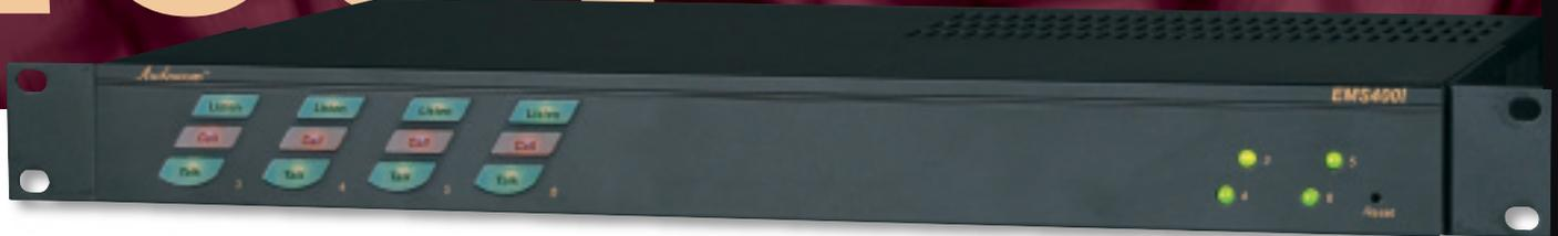
The EMS4001 adds four powered intercom channels to an MS2002 or US2002 Master Station. It connects to the master station with a supplied patch cord. Then, you simply plug it into any AC power outlet from 100 to 240 volts, connect intercom stations to the back panel, and you're ready to communicate on four more channels using the master station microphone and speaker (or headset). The EMS4001 fits in a standard 19-inch equipment rack and is 1 rack unit high.
