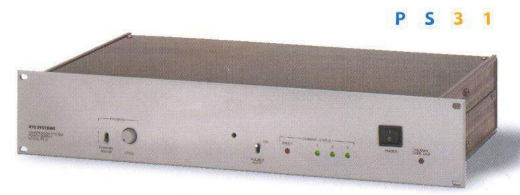
System power supply. Provides three independent powered output channels at 32VDC up to 1.5 amps, program audio inputs and full system status indicators. Features unique circuitry that protect outputs from short circuit conditions with automatic and instantaneous recovery when short is removed. Powers an average of 15 stations per channel for a total of 45. Packaged in a 2 RU by 1 rack all metal housing with a verity of output connectors for multiple-channel configurations.
