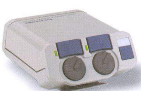
Two channel, binaural, portable beltpack headset station. Features a user programmable microprocessor assisted interface for the highest degree of flexibility and versatility. Allows stereo (split-feed) or mono operation. Includes individual talk/listen buttons, program input with level adjust, A4F/A5F headset connectors, remote mic off feature and call light in a rugged, high impact polycarbonate case.
