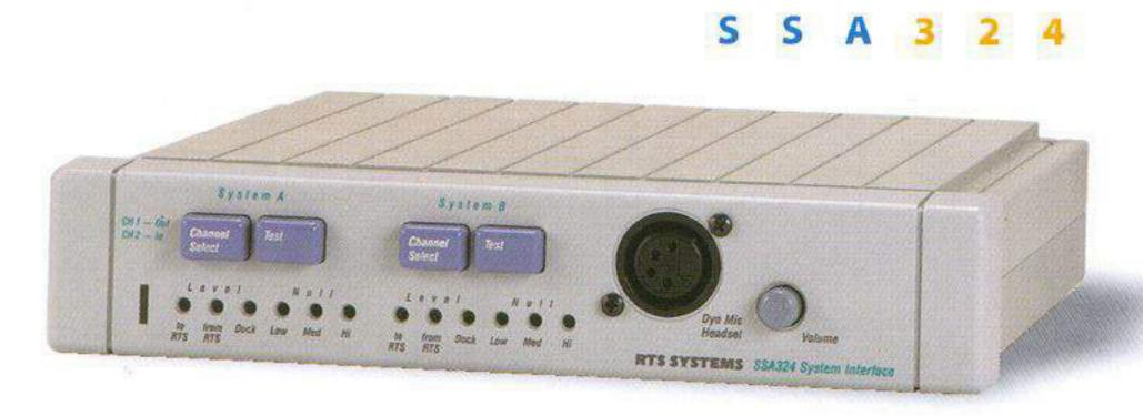
Provides 2 independent channels of 2 wire (TW) to 4 wire hybrids in a 1/2 rack wide by 1 RU package. The TW interface is suitable for balanced and unbalanced systems, allowing RTS party line systems to interface to virtually ANY party-line intercom system in use today. Features system to system level, duck and null adjusts with front panel headset connector for use during setup. Option card allows translation of call lights and two-way radio interfacing.
