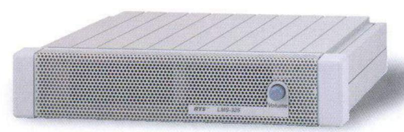
Line monitor speaker station. Part of RTS's unique modular packaging system. Features a full range 5 Watt speaker and power amp, dual channel inputs from TW or separate program inputs and volume control. Packaged in 1/2 rack by 1 RU metal housing for added durability and magnetically shielded for use near video monitors.
