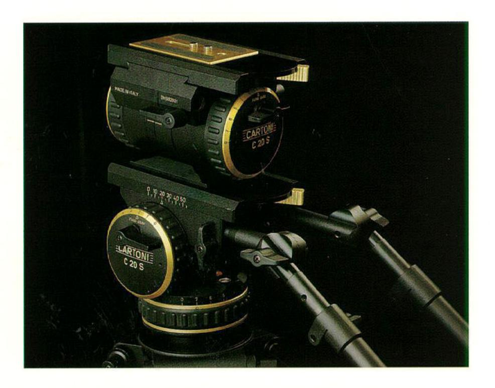
The award-winning **CARTONI** fluid damping modules as well as the spring type counterbalancing system integral to both **C20 S** and **C40 S DUTCH**, provide respectively 7 steps of drag plus "0" and 7 progressive spring tension settings.
